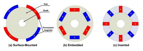
Fig.1.2: Rotor Magnets Cross-Sections
