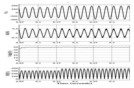
Fig5.7: Input Voltage, Input current, Dc link voltage and capacitor filter voltage at input supply voltage from 220V to 270 V and converter output voltage of 48V
