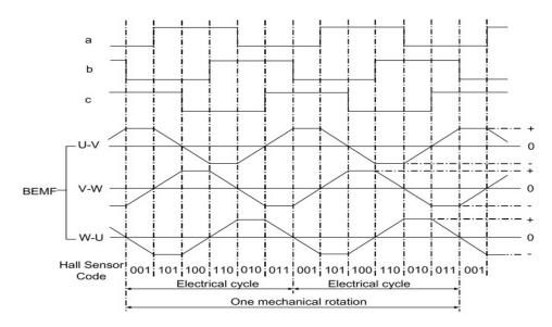
Fig.1.5: Hall Sensor versus BEMF
