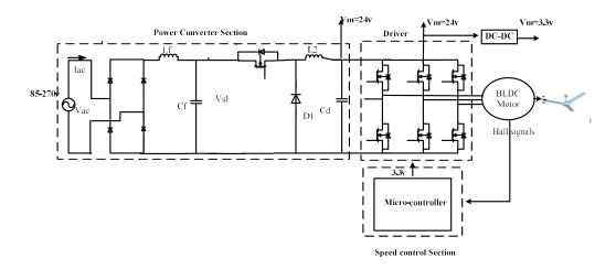
Fig.4.3: Circuit diagram of working of BLDC Motor FAN
