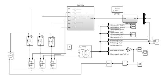
Fig.3.2: MATLAB simulation of speed control of BLDC Motor
