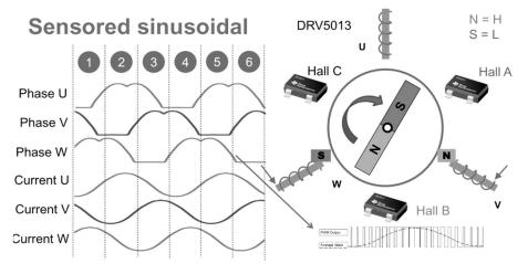
Fig.1.8: Sensored Sinusoidal Control
