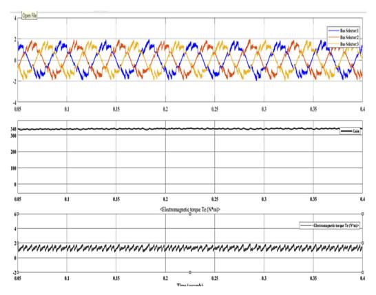
Fig.4.12: Current, Speed and Torque
