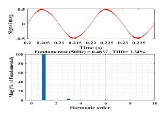
Fig. 5.9: THD in supply current (RMS) at a supply voltage of 270V.
