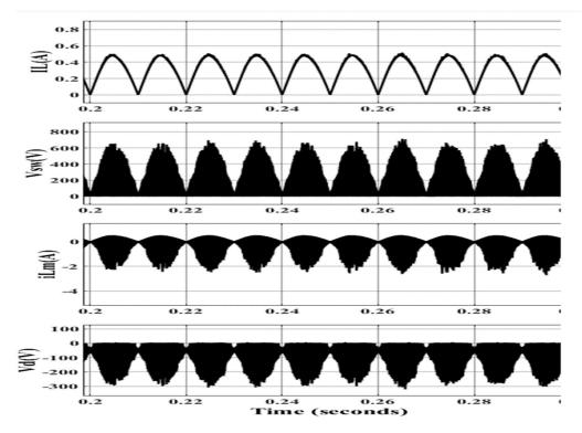
Fig.5.4: current in input side inductor of converter, voltage across switch, current in transformer winding and voltage drop across diode at input supply voltage of 220V and converter output voltage of 48V
