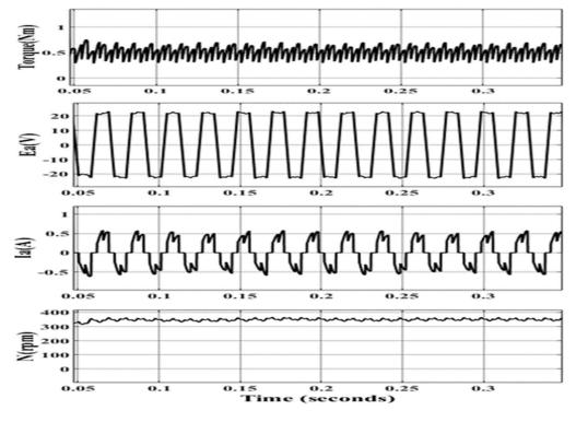
Fig.5.8: performance of ceiling fan under the dynamic condition varies input supply voltage from 220V to 270V at converter output voltage of 48V
