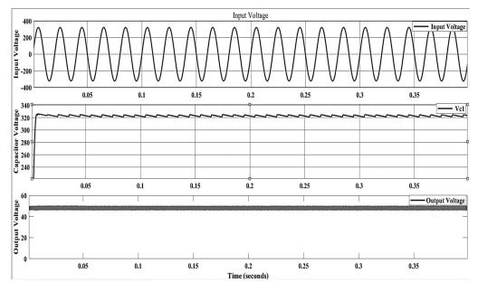
Fig 4.10: Input supply, capacitor voltage and converter output voltage
