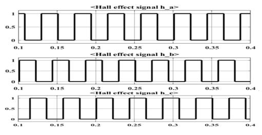
Fig.3.5: Hall-sensor waveform
