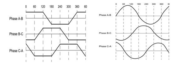
Fig 1.3: Trapezoidal and Sinusoidal stator windings
