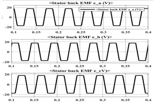
Fig.3.3: BEMF waveforms
