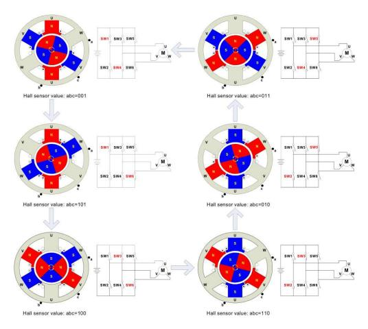
Fig.1.4: Three-Phase BLDC Motor working
