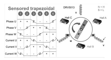
Fig.1.7: Sensored Trapezoidal Control
