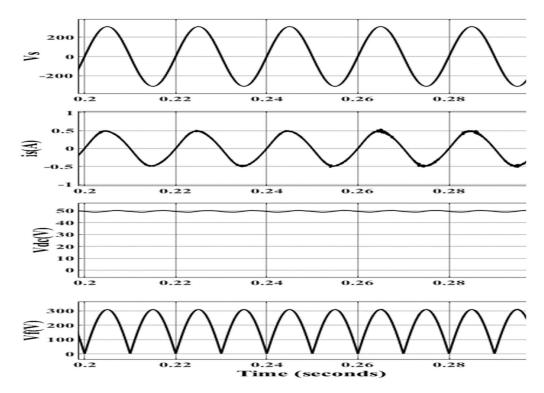
Fig.5.3: Input Voltage, Input current, Dc link voltage and capacitor filter voltage at input supply voltage of 220V and converter output voltage of 48V
