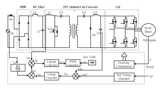
Fig.5.1: A BLDC Motor drive fed by a PFC Isolated Cuk converter in CCM (using a current multiplier approach).
