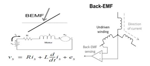
Fig.1.6: BEMF Detection Method
