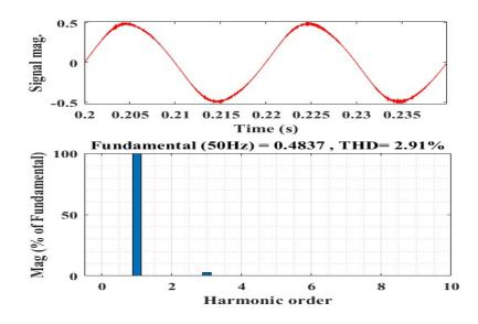
Fig.5.6: THD in supply current (RMS) at a supply voltage of 220V.
